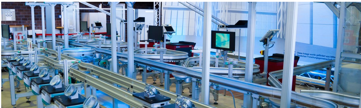
Figure 4.5.1: Cyber-physical platform as prototype for automotive assembly.
